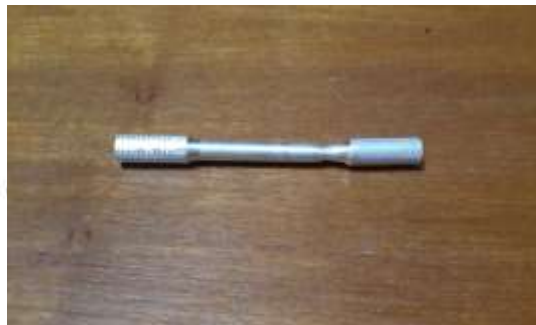
Figure(2) Tensile test specimen (all dimensions in mm) according to ASTM A370 specification
