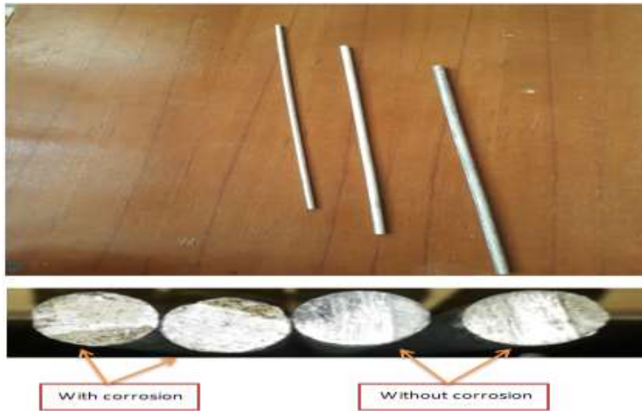
Figure:(7) the specimens with pitting corrosion
