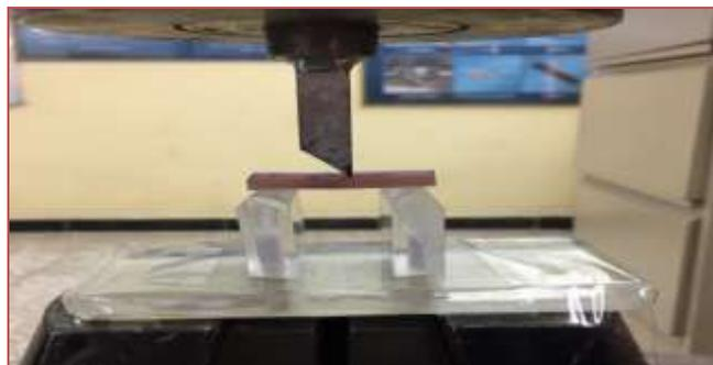
**Figure (13): The max.shear test machine.**
