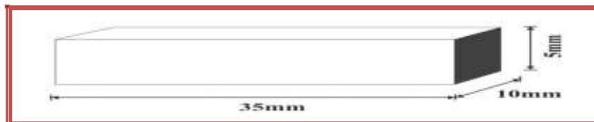
**Figure (12): Schematic Specimen for Standard Specimen of max.shear test .**
