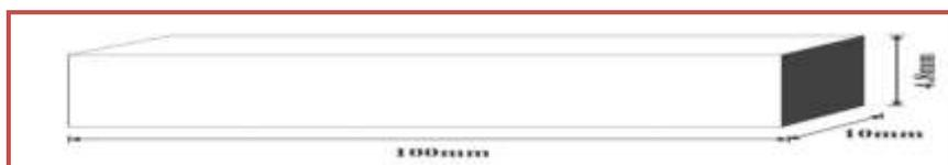
Figure (4): Shows the standard dimension of specimens
