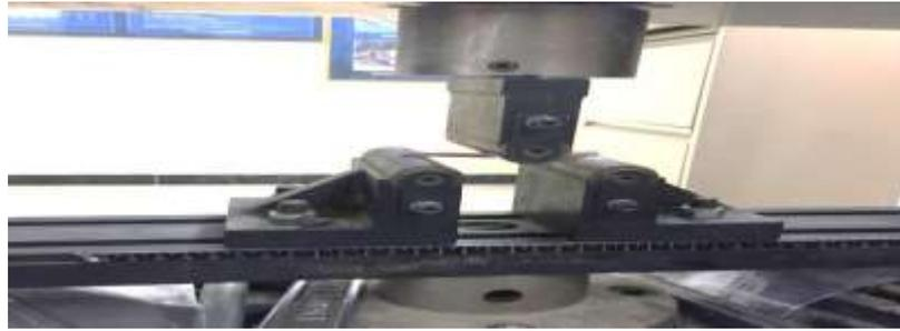
Figure (5): The flexural test machine .
