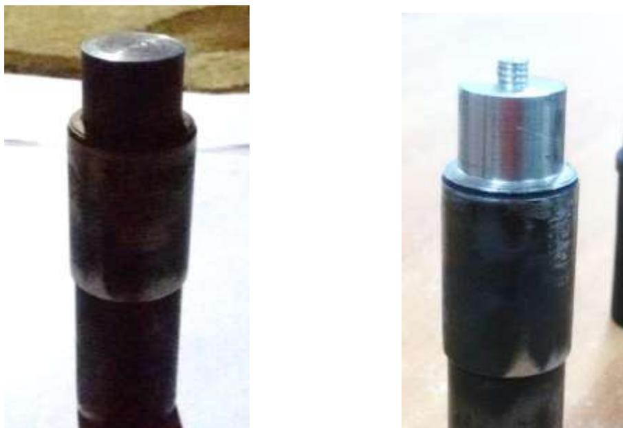
**Figure (1):**Shows (a) FSP tool (b) pin-less tool.
