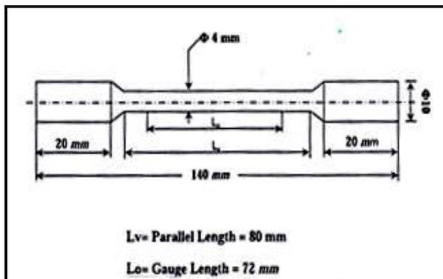
Fig.2. Standard specimen of tensile test [13].
