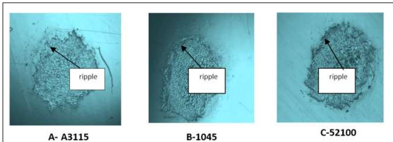
Fig. 7. Photomicrographs of the specimens as after treated by laser showing the ripples .
