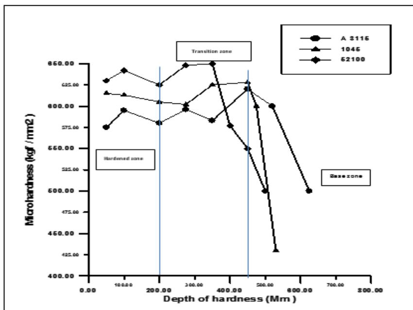
Fig.6. Relationship between microhardness and the depth of hardening of three alloys after laser surface treatment.
