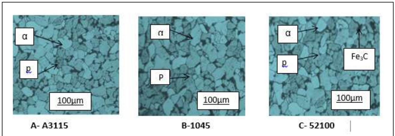
Fig.4. Photomicrographs show the microstructure of the specimens as - received with 300X asa magnification.
