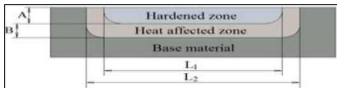
Fig.1.Different zones of laser transformation hardening [7] .
