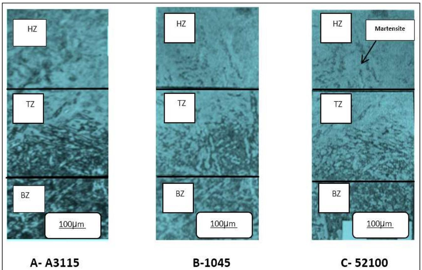
Fig.5. Photomicrographs of the specimens treated by laser showing the different hardened zones with 300X as a magnification.
