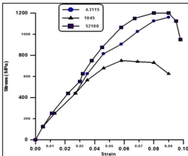
Fig.3.The relationships between stress– strain for the specimens as- received.
