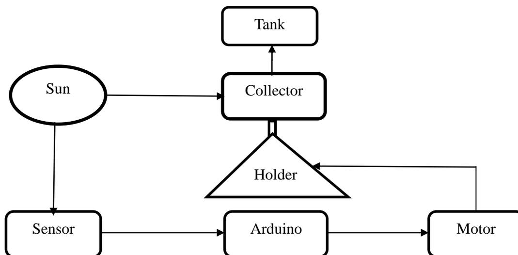
**Fig. (1)** Block diagram of solar collector system model
