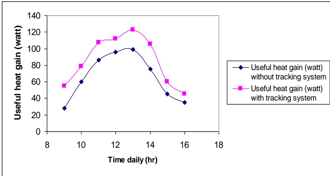
Fig. (11) Useful heat gain of solar collector without and with tracking system
