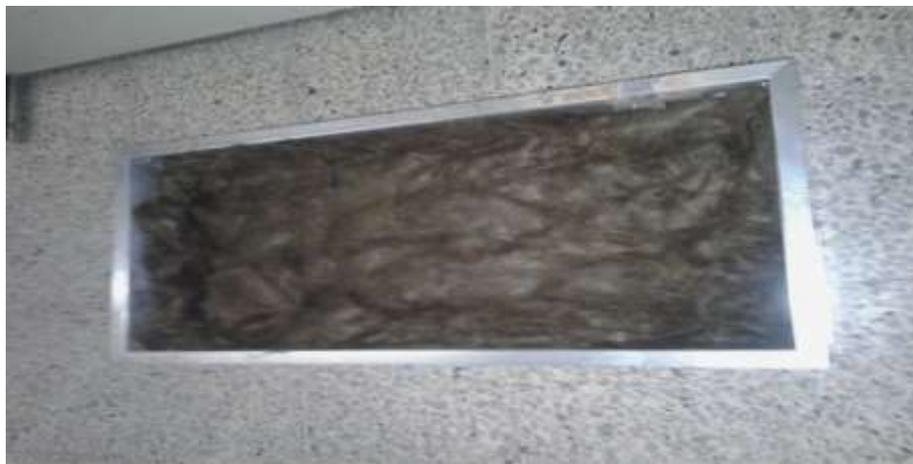
**Fig. (3)** Thermal insulation between the bottom of the frame and the lower side of the absorber plate.
