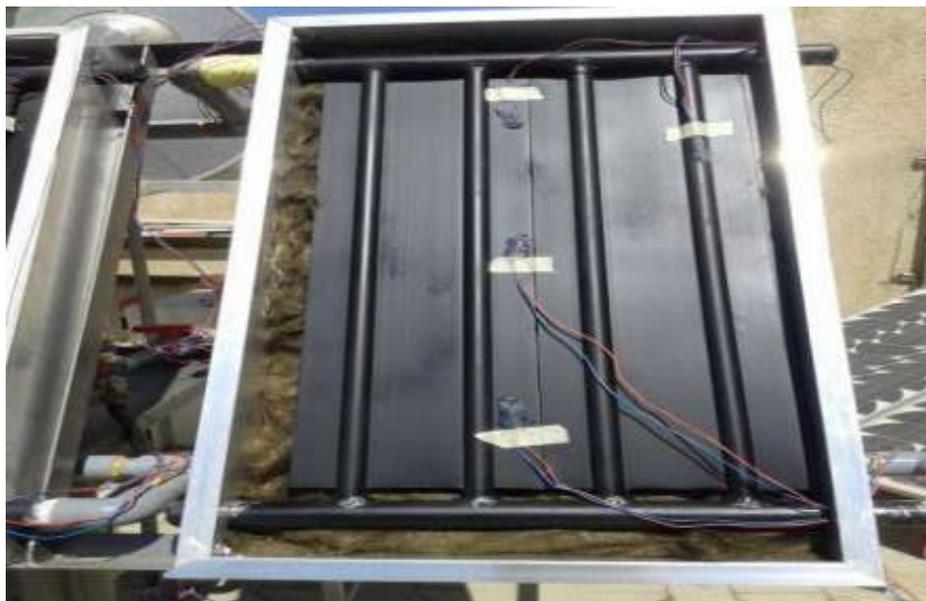
**Fig. (5)** The final form of solar collector parts assembly
