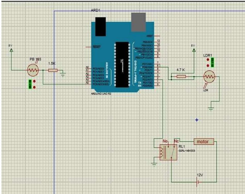
Fig. (7) Electrical circuit of solar tracker system
