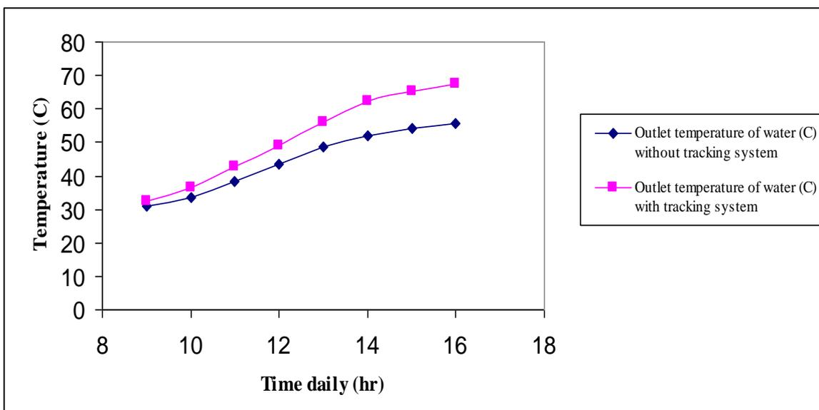
Fig. (10) Outlet temperature of solar collector without and with tracking system
