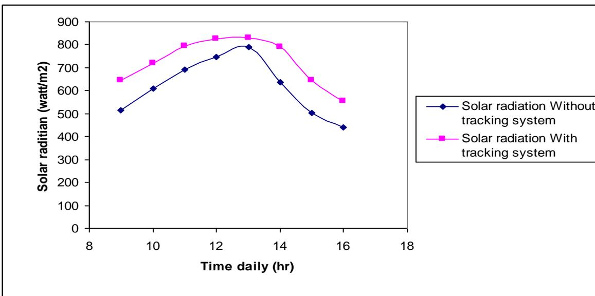
Fig. (9) Solar radiation without tracking and with tracking system in 2<sup>nd</sup>, 3<sup>th</sup> of Jun 2015
