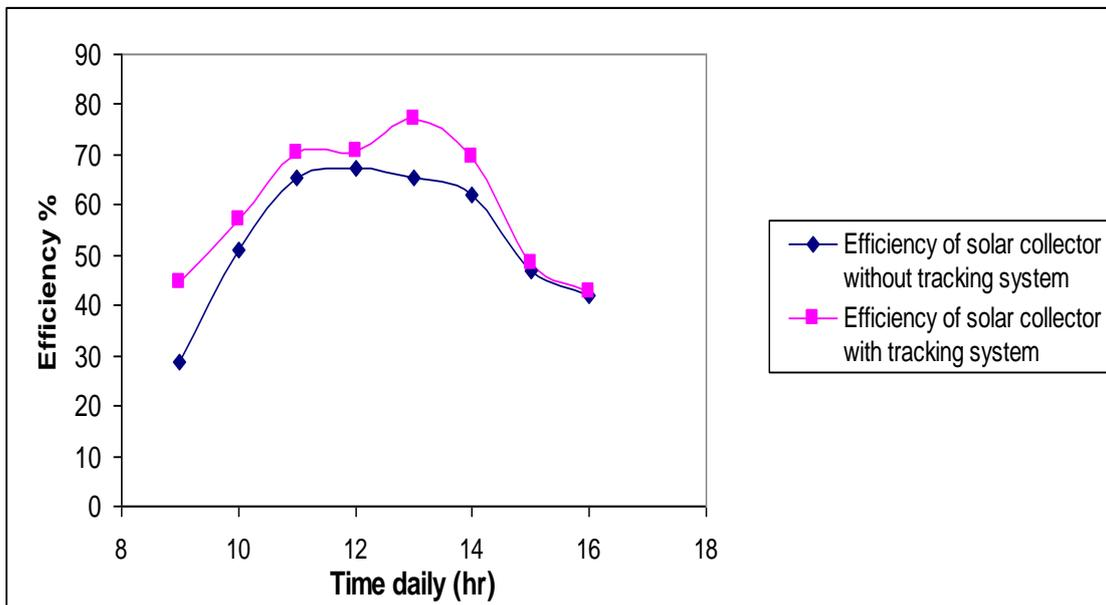
Fig. (12) Efficiency of solar collector without and with tracking system
