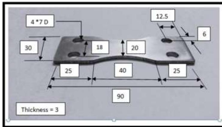
**Fig.1,** Geometry of fatigue specimens dimensions are in millimeter
