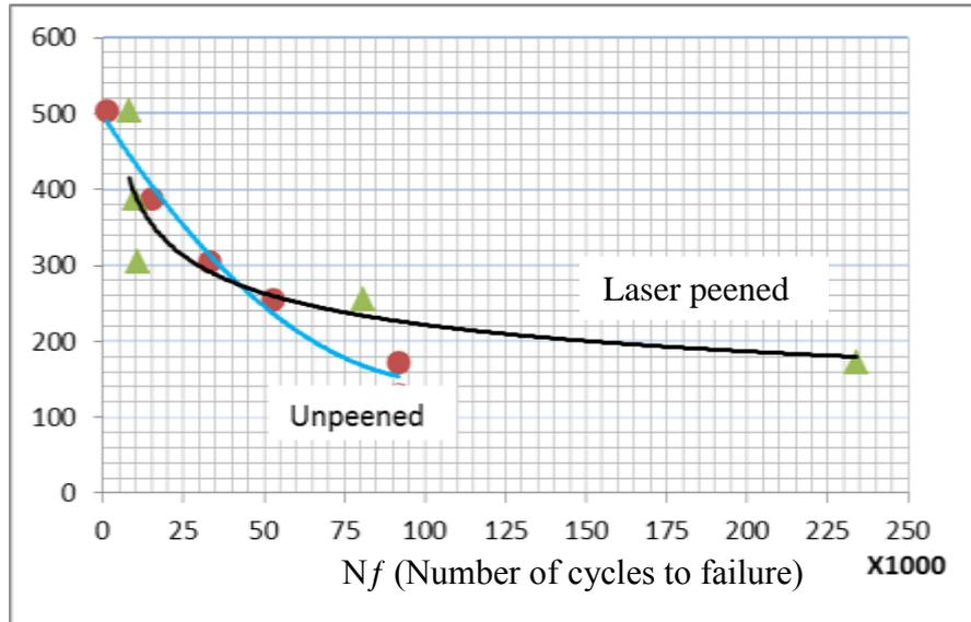
Fig.4: S-N curves at constant load for laser peening
