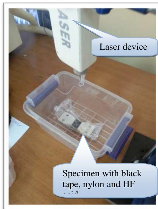
**Fig.3** specimen applied under laser power
