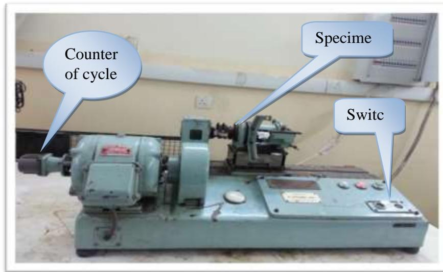
**Fig 2.** Avery fatigue bending machine
