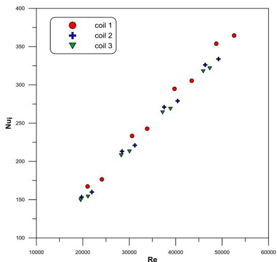
**Fig. (5) :** Inner Nusselt number versus Reynolds number for different Curvature ratio
