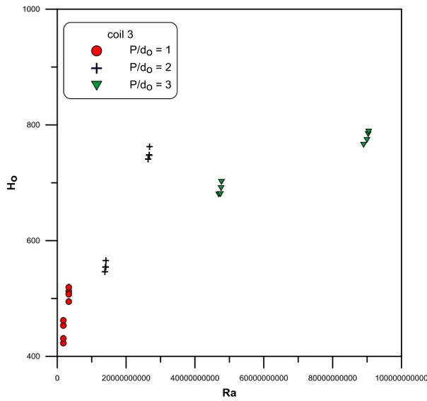
**Fig. (9) :** Effect of the coil pitch on the outer heat transfer coefficient for coil 3
