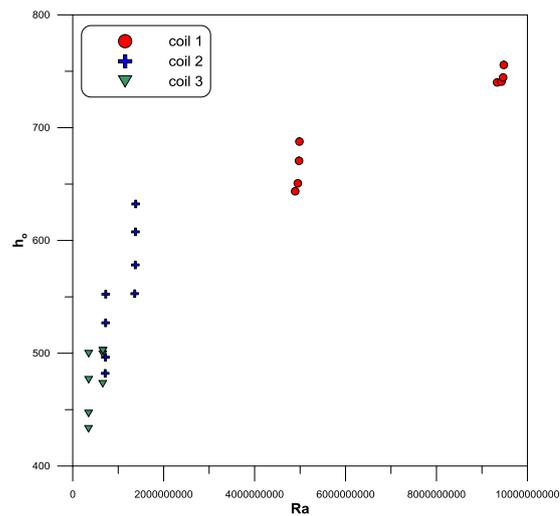
**Fig. (6) :** Outer heat transfer coefficient versus Rayleigh number for different curvature ratio
