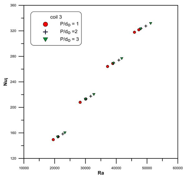
**Fig. (7) :** effect of the coil pitch on inner Nusselt number for coil 3
