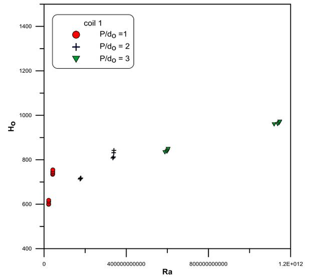
**Fig. (10) :** Effect of the coil pitch on the outer heat transfer coefficient for coil 1
