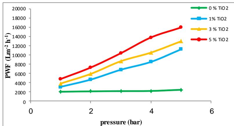
(Fig. 8) : Effect of membrane pressure on the pure water permeation flux of the (Nylon-6 / TiO<sub>2</sub>) nanofiber membrane.
