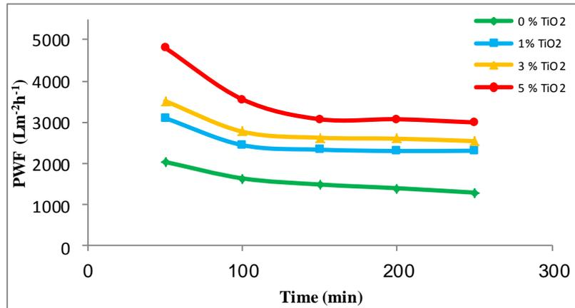
(Fig. 7) : Pure water permeation flux with time of (Nylon-6/ TiO<sub>2</sub>) nanofiber membrane at room temperature and (1 bar) pressure.
