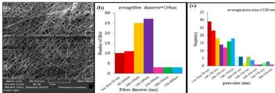
**(Fig. 2):** (a) SEM image of pure (Nylon-6) nanofibers membrane, (b) diameter distribution and (c) pore size distribution .
