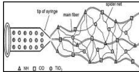
(Fig. 4): Schematic illustration showing the mechanism of (spider-net like structure) formation during electrospinning .
