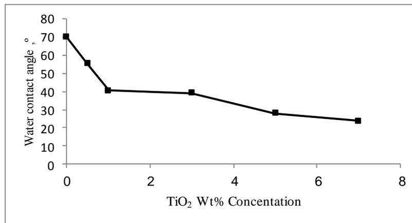
(Fig. 6): Effect of (TiO<sub>2</sub>) addition on water contact angle of electrospun nanofiber membrane.
