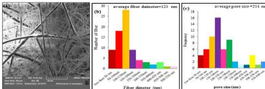
**(Fig. 3):** (a) SEM image of (7% TiO<sub>2</sub>) nanofibers membrane, (b) diameter distribution and (c) pore size distribution.
