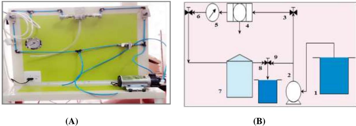
**(Fig. 1):** Pressure cross flow (A) image of filtration system (B) Schematic diagram of the filtration system process. Where 1. Tank for water sample test. 2. Pump. 3. Valve entry. 4. Filter / Module. 5. Pressure gage. 6. Valve out. 7. Open tank for permeate water sample. 8. Tank of rejected water sample. 9. Recycle valve .
