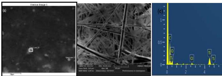
(Fig. 5): (a) Section selected from SEM image (b) SEM Image (c) EDX of (7% TiO<sub>2</sub> / Nylon-6) nanofiber membrane .
