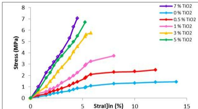
(Fig. 12): Stress-strain curve of (TiO<sub>2</sub>/Nylon-6) with various concentrations.
