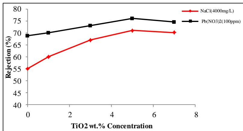
(Fig.9) : Effect of (Nylon /TiO<sub>2</sub>) ratio on rejection of (Pb(NO<sub>3</sub>)<sub>2</sub>) salt and (NaCl) Salt aqueous solutions with initial concentration (100 ppm) and (4000mg/L) respectively, at room temperature and (1 bar) Pressure.
