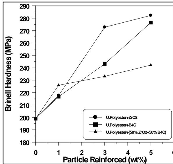
Figure (3) Effect of Particle contents on Hardness.
