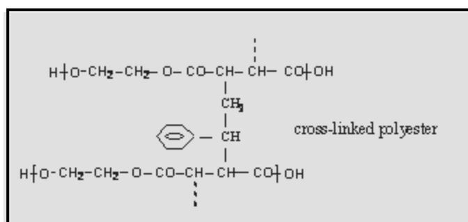
Figure (1): Unsaturated polyester structure.
