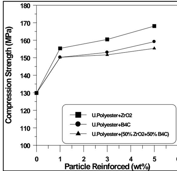
Figure (5) Effect of Particle contents on compression strength.
