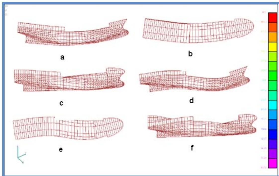
Fig.( 10 ) Trawler beam stress mode shapes
