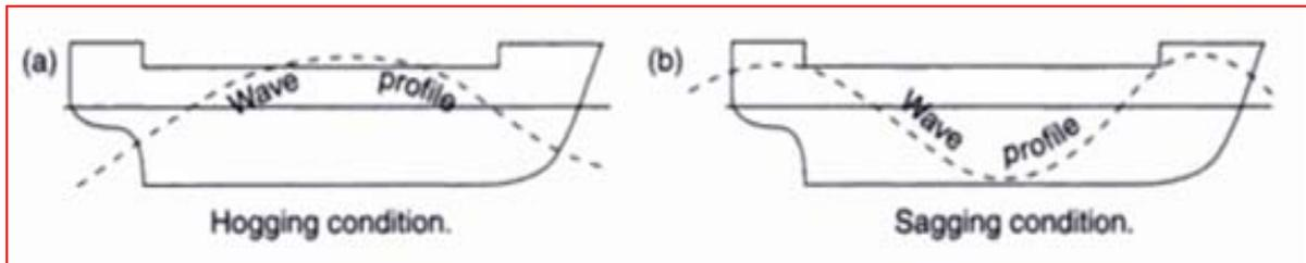
Fig.( 3 ) Ship motion in waves a-Hogging condition (Crest condition)
