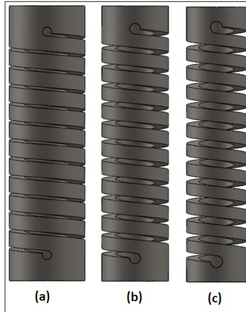
**Figure 5:** Machined spring with different pitch angle (degree)
