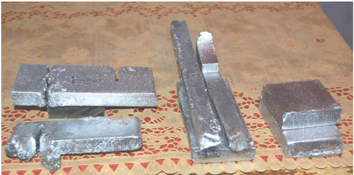
Fig. 5: shows gradual improvement on cut - from left to right – starting with (50) second preheating time (left) to (15) second (right picture). The process curve shown in fig. 4.
