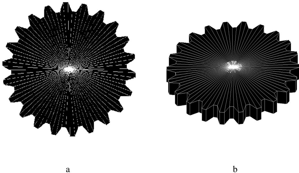
No. of teeth = 22, Tooth Height = 5 mm, Tip Diameter = 61 mm,
