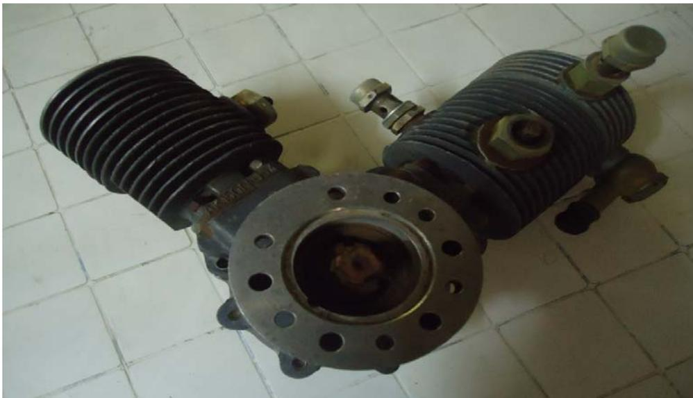
**Fig-2. Reciprocating air compressor ( V-AK 150)**
